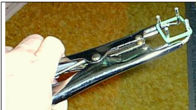
Figure 5. Elastrator tool used to apply rubber rings
